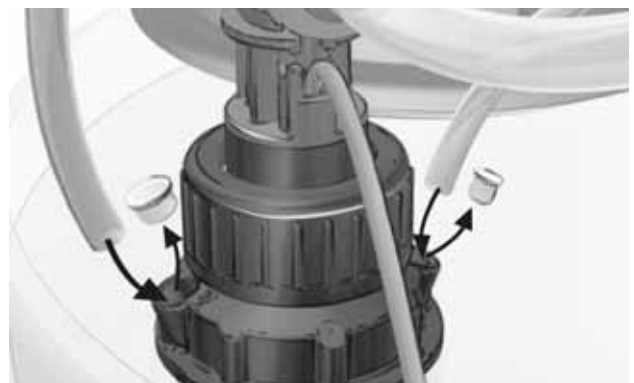
Fig. 12 Suction lance: insert lines into tank connection
